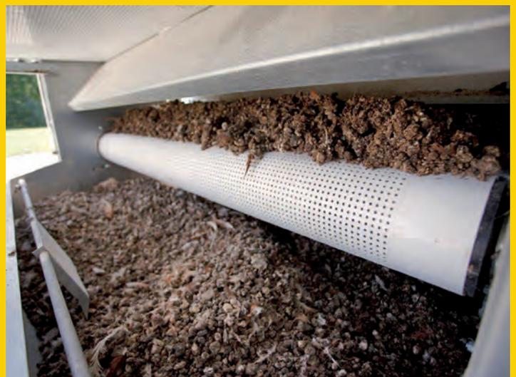
By using fans of pressure first the warm air of the stable will be conveyed into a room and creates there an overpressure. Due to this pressure the warm air of the stable will be pressed through the levels of the drying tunnel and through the manure and passes to the outside. The warm stable air, which was pressed through the manure, dried the manure on the perforated belts.
