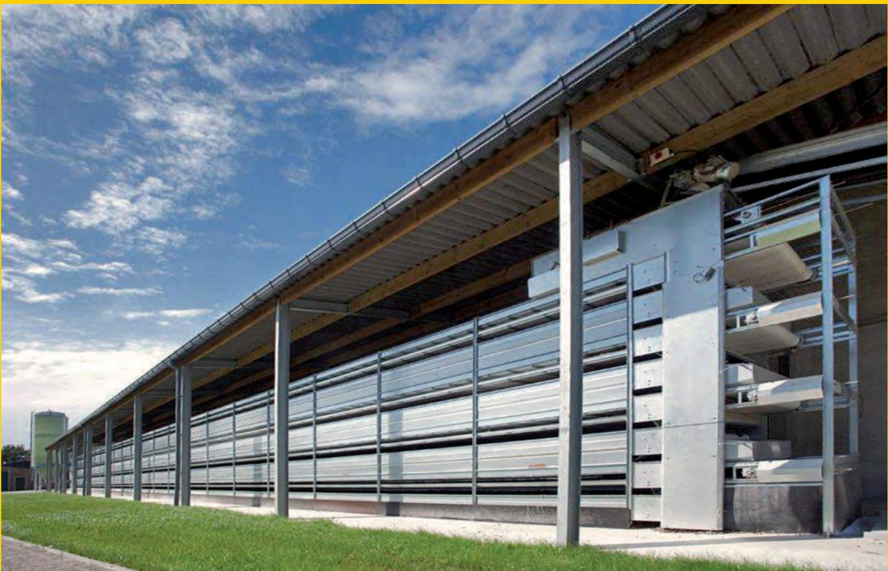
The new Specht-Manure-Drying Tunnel is a developed system of drying manure. Due to the new system there is a significant reducing of ammonia concentration and a drying result of the manure up to 90 % possible.
